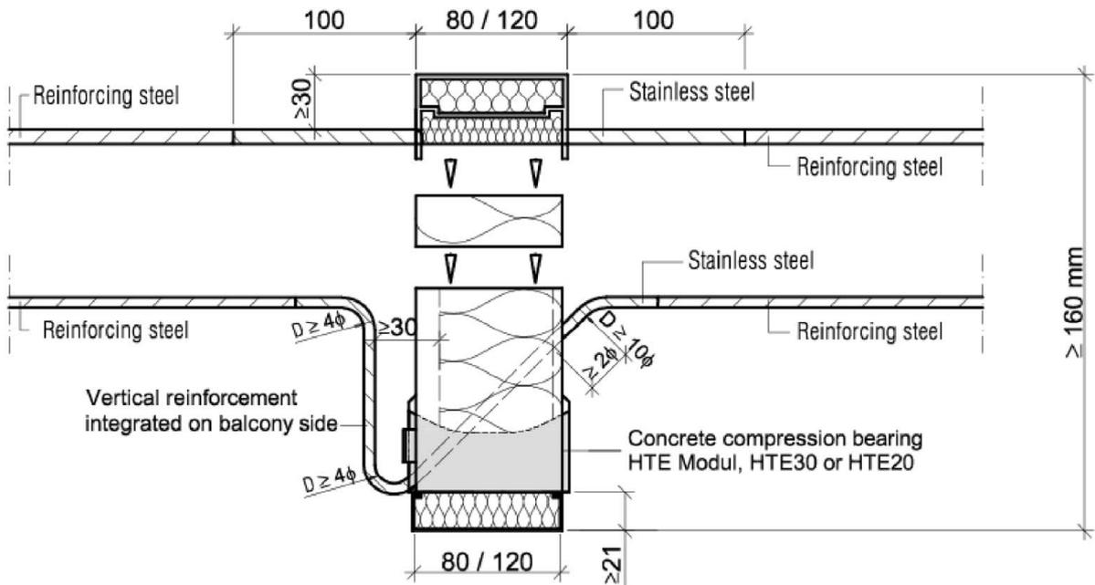
Fig. 19: Example: Schöck Isokorb® type K-F (multi-part variant) with CCE
