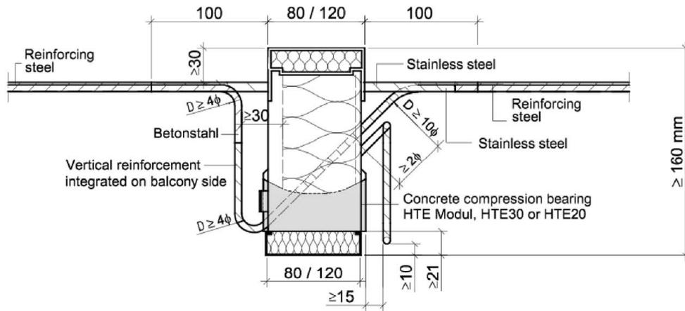
Fig. 41: Schöck Isokorb® type K <sup>1)</sup> with integrated reinforcement stirrups as per Section. D.1.1 and special stirrup
