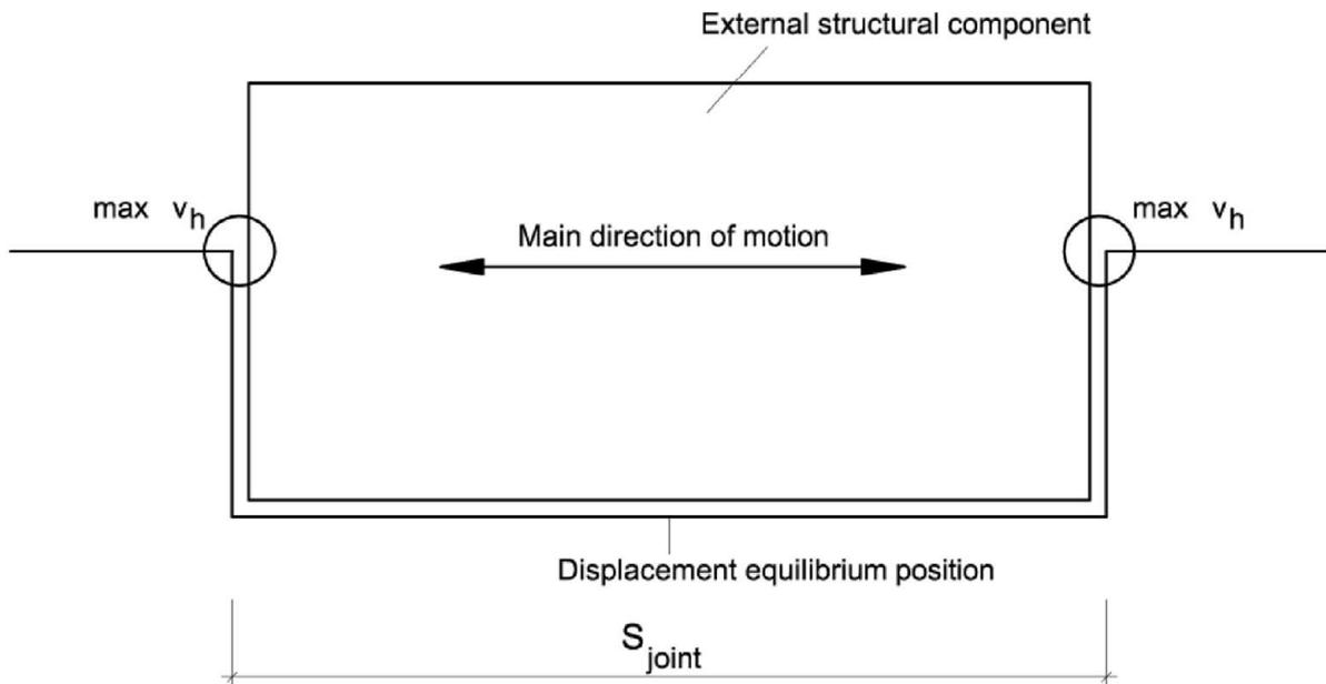
Fig. 15 Installation situation with support on opposite edges
