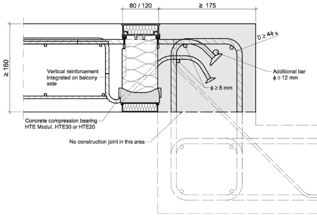
Fig. 22: Schöck Isokorb® type K-O with CCE in installed condition
