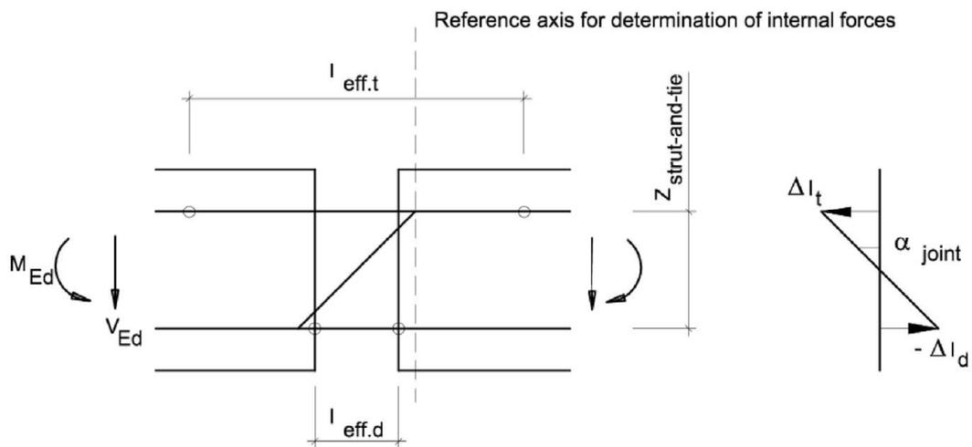
Fig. 52: Model for determining the bending deformation in the joint
