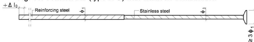
Fig. 14: Tension bar (type K-U) with diameter combination
