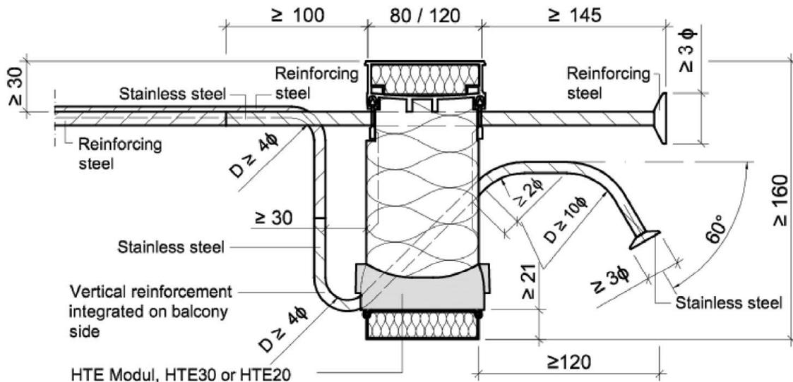
Fig. 23: Example: Schöck Isokorb® type K-U with CCE
