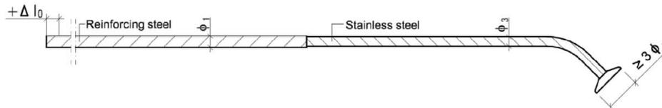
Fig. 13: Tension bar (type K-O) with diameter combination
