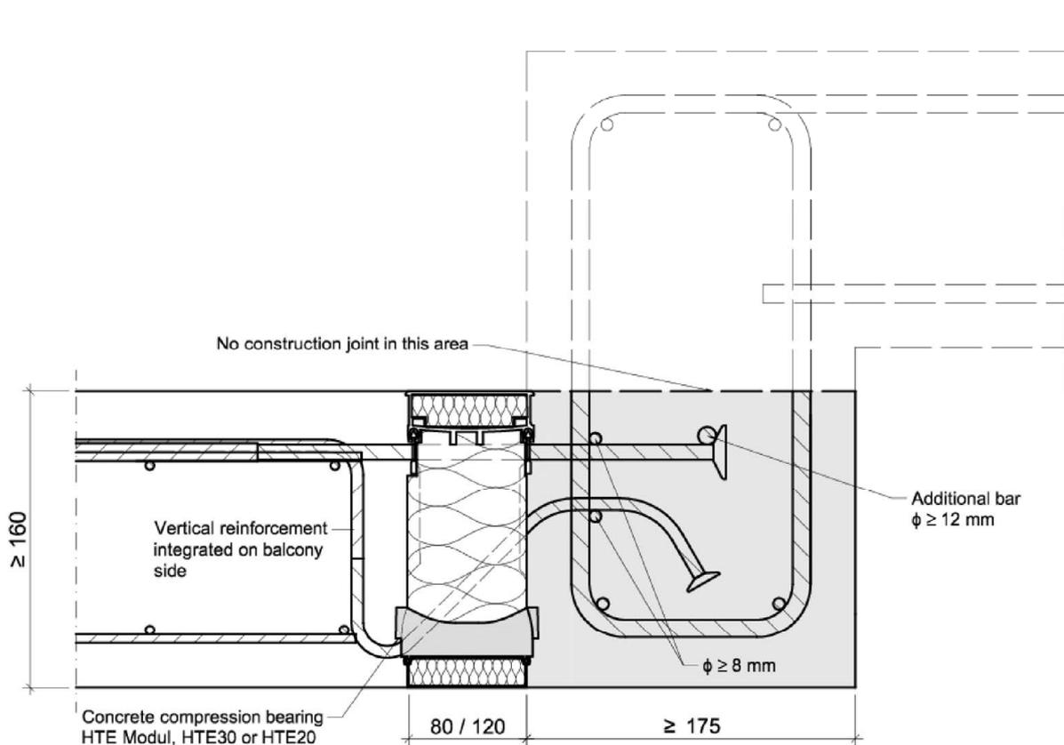
Fig. 24: Schöck Isokorb® type K-U with CCE in installed condition
