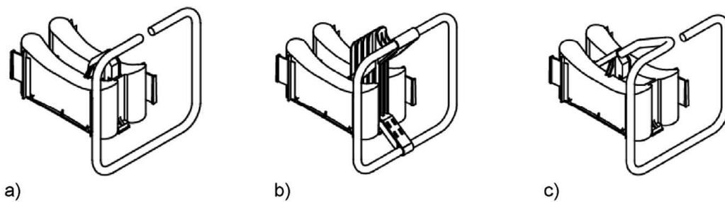
Fig. 43: Concrete compression bearing with special stirrup
