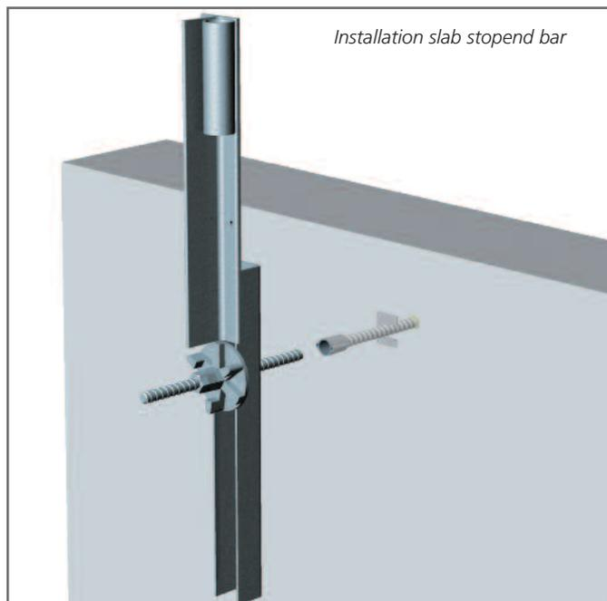
Installation slab stop end bar
