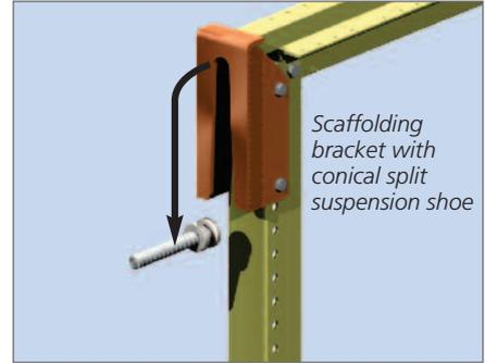
Scaffolding bracket with conical split suspension shoe
