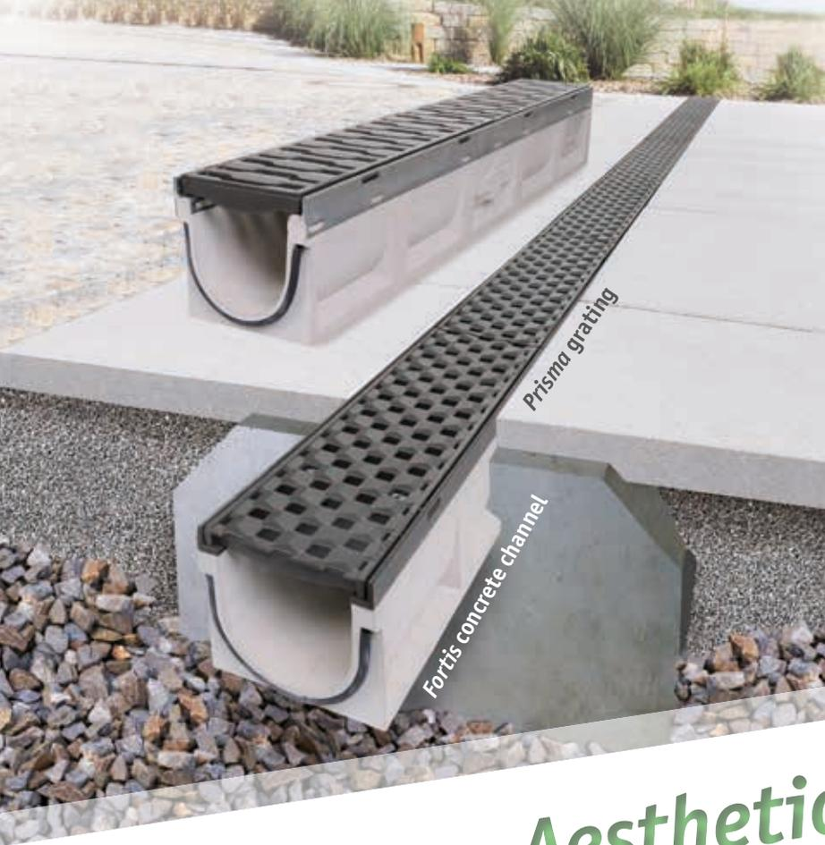
The Fortis concrete channels impress by offering maximum stability despite their low weight. The channels' structure is designed in such a way that they can withstand load class D 400 once embedded in a standard concrete foundation. The same applies to the drainage and point drainage units.
