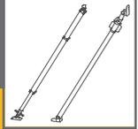
Spindle element with combination end hinge, extended at least 25 mm, that means min. length of 1120 mm, limitation through contact of the spindle at the end hinge. At length of 1095 to 1120 mm contact of the clamping nut to the concrete.
