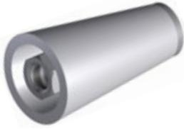
The Steel-Plastic Cone with steel core is an alternative to Steel Cones. Its field of application and its load bearing capacity are identical to those of Steel Cones. The Steel-Plastic Cone can be removed from the formwork more easily due to its larger cone inclination and the plastic sheathing. Furthermore, the remaining hole can be closed much better and easier using the matching concrete plug.
