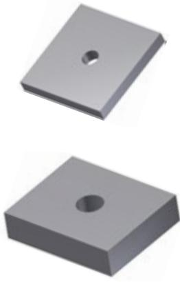
Flat Plates are used for timber or steel walings in conjunction with a winged nut or a hex nut for load transfer. Load capacity depends on the contact area, the admissible bearing pressure and the threadbar that is used.
